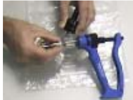
Re-tighten the needle nut.
