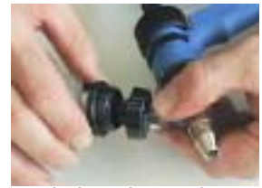
Insert bottle attachment and rotate bottle locking ring to secure.
