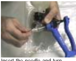
Insert the needle and turn clockwise to tighten.
