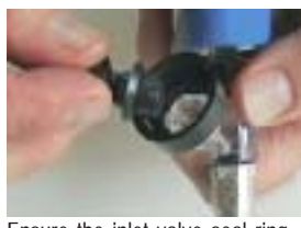
Ensure the inlet valve seal ring and spring are in place.
