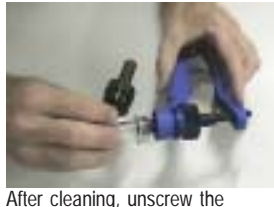
After cleaning, unscrew the cylinder anticlockwise and remove the top of the bottle attachment.
