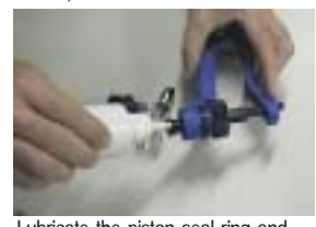
Lubricate the piston seal ring and re-attach the cylinder. Ensure the cylinder is aligned with the body of the instrument.
