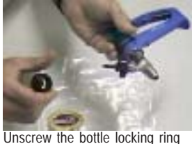
Unscrew the bottle locking ring and remove the bottle.
