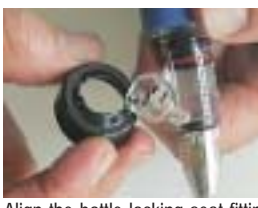
Align the bottle locking seat fitting with the grooves on the cylinder.
