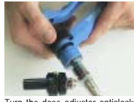
Turn the dose adjuster anticlockwise to decrease the dose, clockwise to increase the dose.
